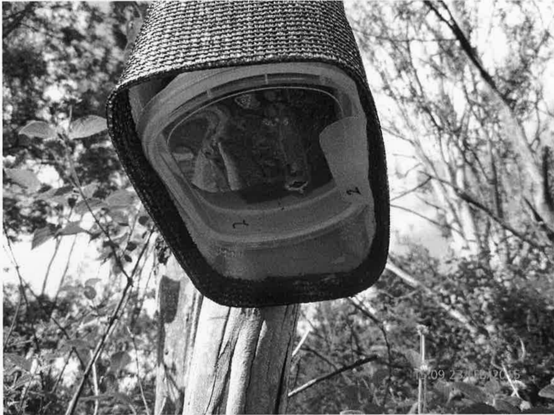
Figure 5. A frog call recording unit, set at a water body site (Source: Melissa Tully, 2016)
