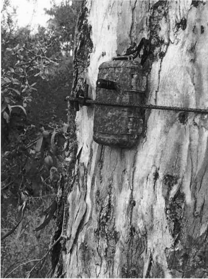
Figure 6. Anabat unit set on tree trunk, 1-2 m from the ground, in a potential flyway at a Cumberland plain woodland site (source: Melissa Tully).
